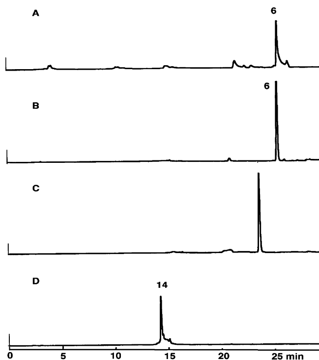
FIGURE 2. Reversed-phase HPLC chromatograms (detection at 260 nm) of (A) the crude mixture of the 5'-protected aminoxy oligonucleotide 6 , (B) the purified 5'-protected aminoxy oligonucleotide 6 , (C) the crude mixture of oxidation of 6 , and (D) the crude mixture of cyclization of 6 leading to 14 .
